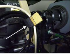
Notice the BNC lead is strapped down for strain relief.
