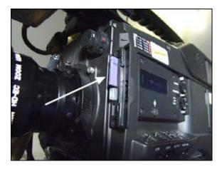
Once the camera operations have been set-up ie: graticules/display functions/frame rate/shutter speed etc, these should be recorded to the memory stick and should also be backed up. The functions should also be written down on paper for further safeguarding.
