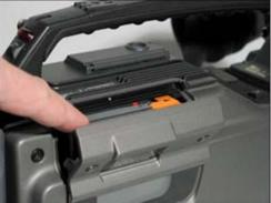
10. WARNING: The camera should be powered with 12 Volt DC only. 24/30V Batteries will blow the camera up!
