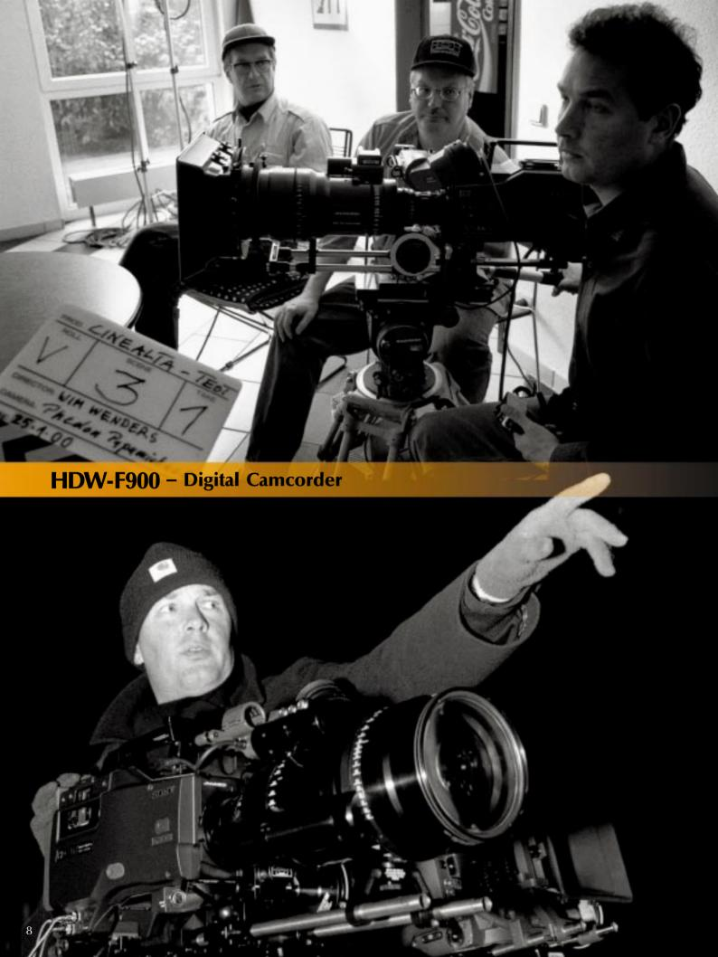
The HDW-F900 digital HDCAM camcorder combines a 3-CCD HD color digital camera, where each RGB imager has 1920 (H) x 1080 (V) sensors, with an HDCAM compact digital 1/2-inch cassette recorder. These superb new CCDs, a 12-bit A/D converter and advanced DSP processing combine to make a camcorder ideal for digital cinematography. The introduction of new techniques of HD signal processing improves the image quality even further while also simplifying the overall setup operation.
