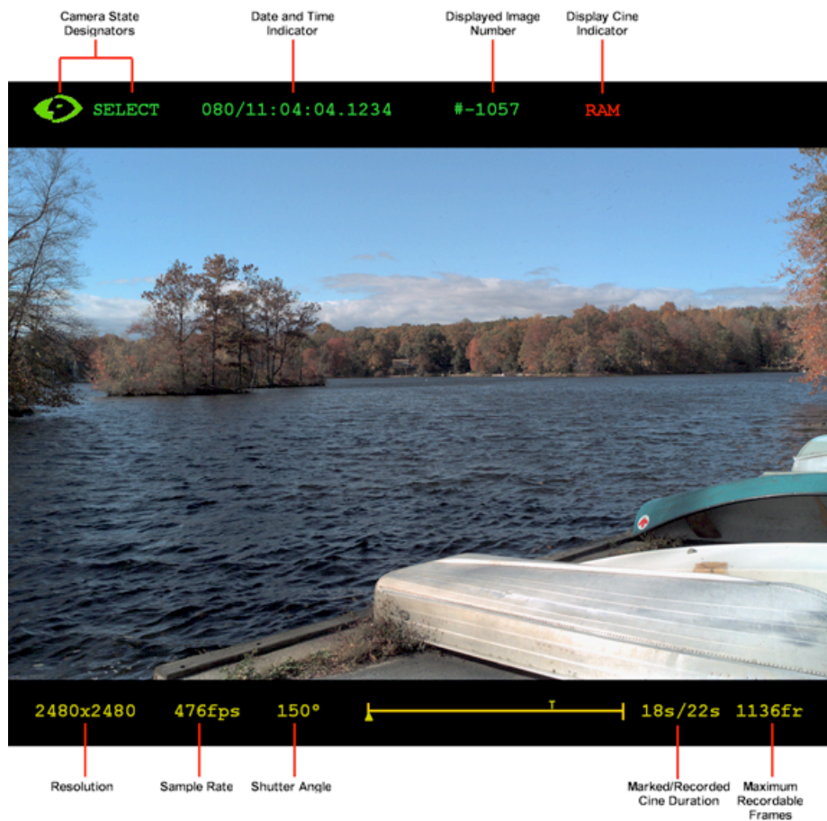
SELECT Mode Display Screen without an attached Phantom CineMag
