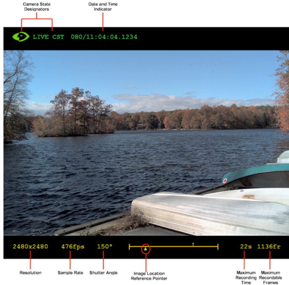
LIVE CST Display - Cine Stored Mode without an attached Phantom CineMag
