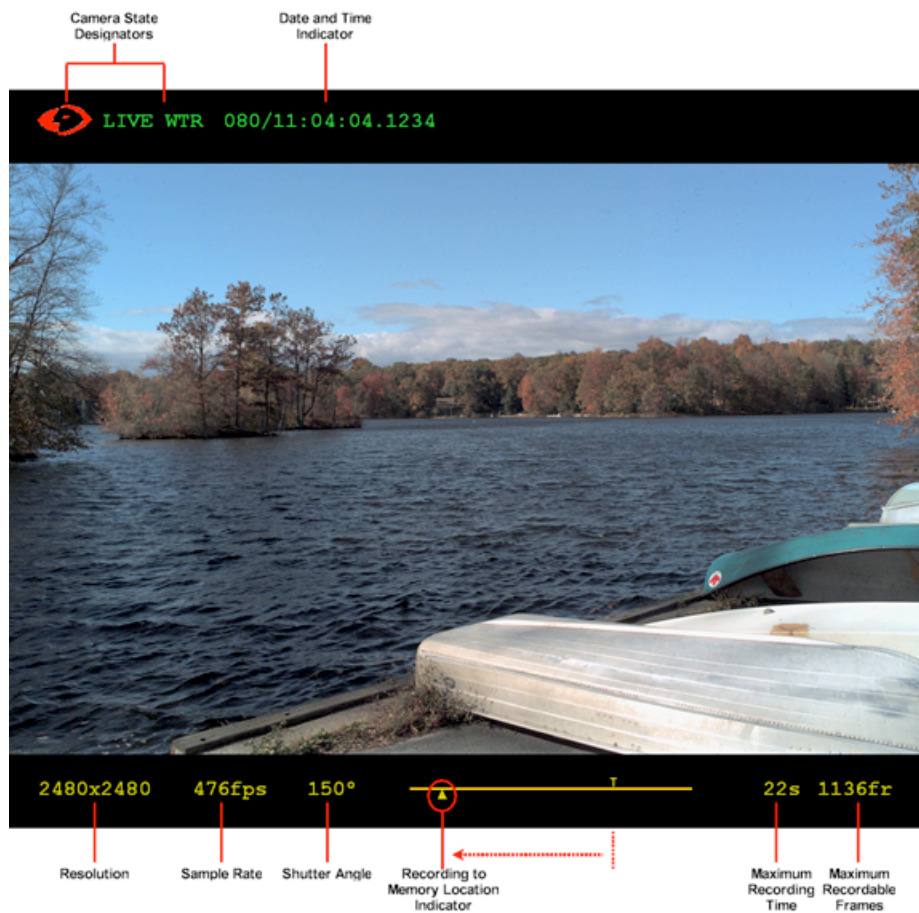
LIVE WTR Display - Recording, Waiting for Trigger Mode without an attached Phantom CineMag
