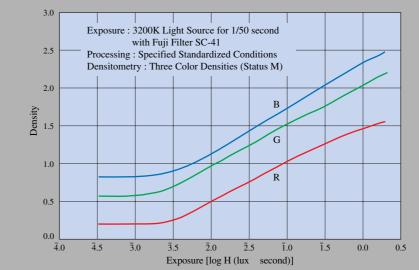
In order to simulate conditions closest to practical use, exposure was made under a 3200K light source, through a Fuji SC-41 ultraviolet absorbing filter. Processing was carried out under standard conditions and the three color densities (status M) were measured. The results of measurements are plotted as characteristic curves.
