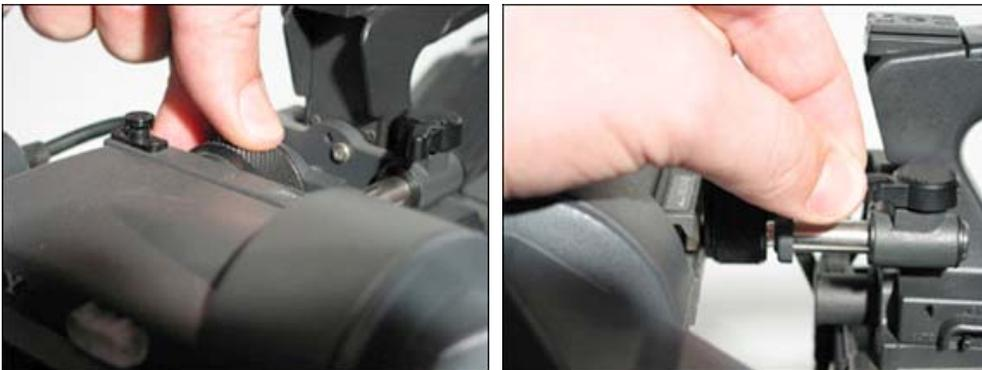
3. Check mounting screws on the viewfinder are tight. Check the lock off for play...there is always a bit.
