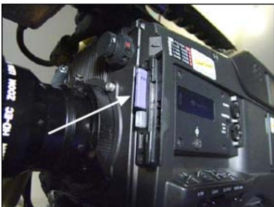
Once the camera operations have been set-up ie: graticules/display functions/frame rate/shutter speed etc, these should be recorded to the memory stick and should also be backed up. The functions should also be written down on paper for further safeguarding.
