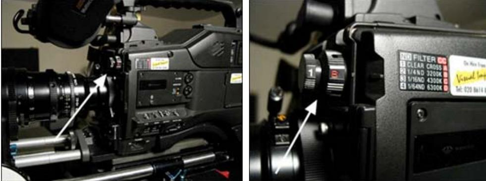
The default colour temperature of the CCD is 3200K.
