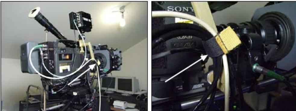
*Notice the BNC lead is strapped down for strain relief.*
