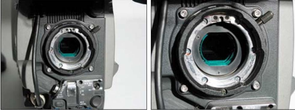
2. Check CCD filter (behind lens mount) is clear of dust, finger marks or scratches.
