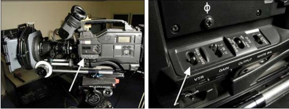
It's advisable to use the camera in the save position. This will save the head drum from constantly running on the tape in the same place while you set-up. It can also avoid head clogs and the save function will save on battery life. Save needs approximately 3.5 seconds for run up to speed.
