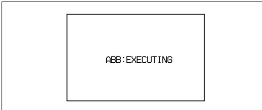
The black balance adjustment ends in a few seconds with the message “ABB:OK” and the adjustment setting is automatically stored in memory.
