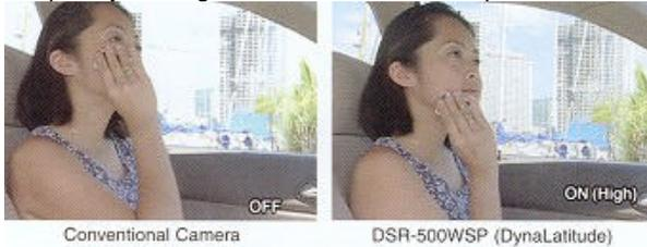
distribution. The DynaLatitude brings a new dimension to the technologies such as Dynamic Contrast Control (DCC) that control the dynamic range of video signals. The DynaLatitude™ feature optimizes video level distribution based on video signal histograms in order to utilize the limited dynamic range of the video signal standard.
