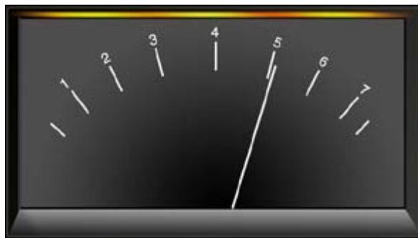
Peak Programme Meter: showing PPM 5 which is equal to +4Dbm's
