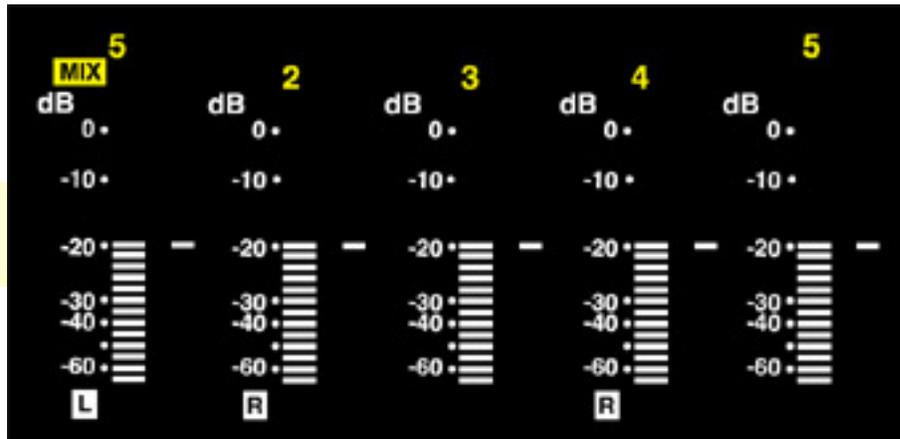
Digital VTR full scale meters; showing -20Db's
