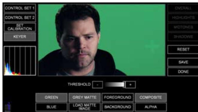
The RGB difference keyer works on a „threshold“ principal, where the lower the threshold, the more green or blue is keyed out. The general workflow is that the user picks the screen color using the GREEN or BLUE buttons, and then reduces the threshold until a proper key is made.
