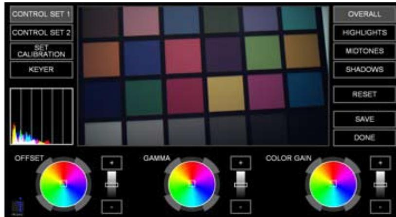
The IRIDAS color-correction control panel is split into three main areas: 1) the control panel modes and metering indicators, 2) file management and luminance separation controls, and 3) the control surface itself.
